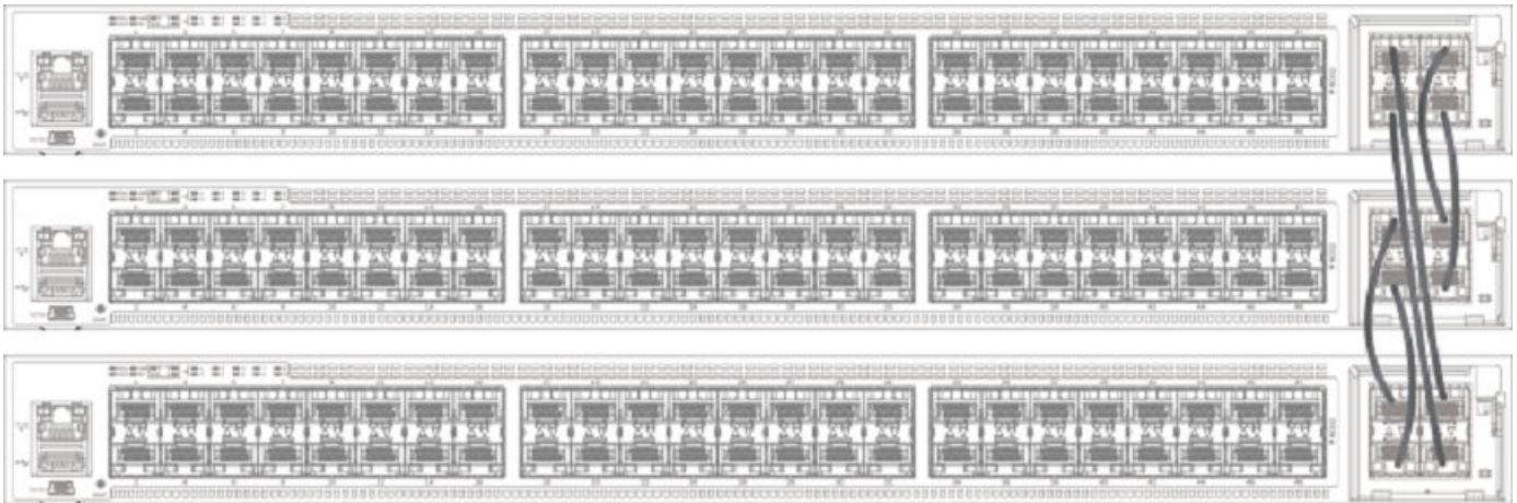
FIGURE 23 ICX 7450 4 X 10-Gbps ring using stacking trunks
